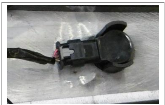
Figure 9: Parking sensor fitted to Protection Bar
