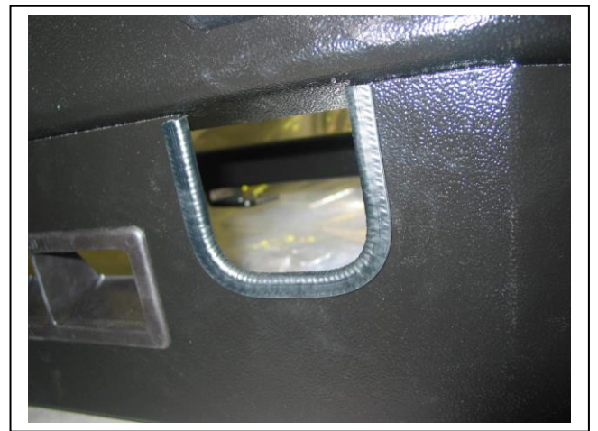
Figure 8: 3mm clip lock trim fitted
