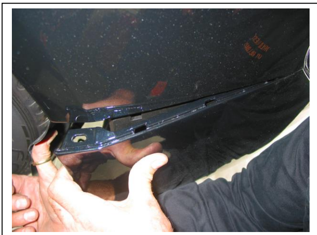
Figure 1: pull bumper rearward and out to release.
