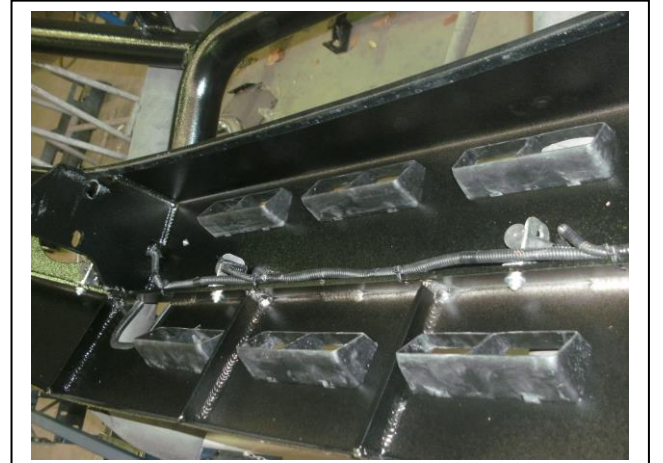
Figure 10: Wiring in rear of Protection Bar
